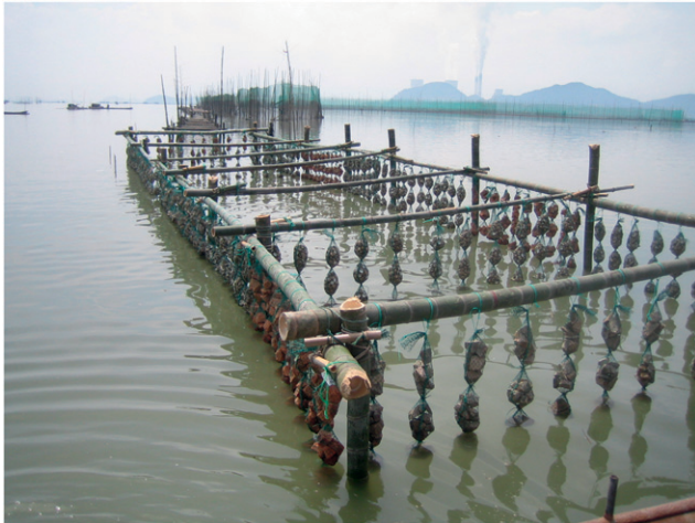
Figure 2. The experimental bamboo frame and substrate bags within the intertidal zone adjacent to active oyster aquaculture farms.
